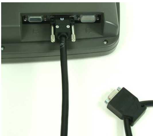
Diagr. 3-8 BASIC - Terminal with MFG connecting cable and connection for the basic equipment
